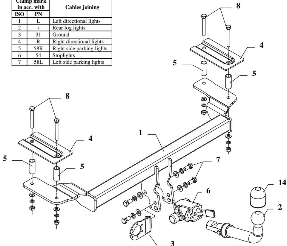
This towbar is designed to assembly in following cars: **FORD FIESTA, 3-5 doors** and **MAZDA 121 JASM/JBSM, 3 doors**, both produced since 02.1996 till 12.2001, catalogue no. **C002A** and is prepared to tow trailers max total weight **950 kg** and max vertical load **50 kg**.
