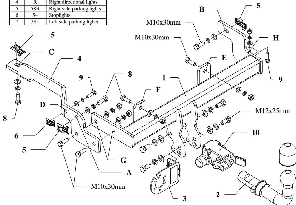
This towing hitch is designed to assembly in following cars:
