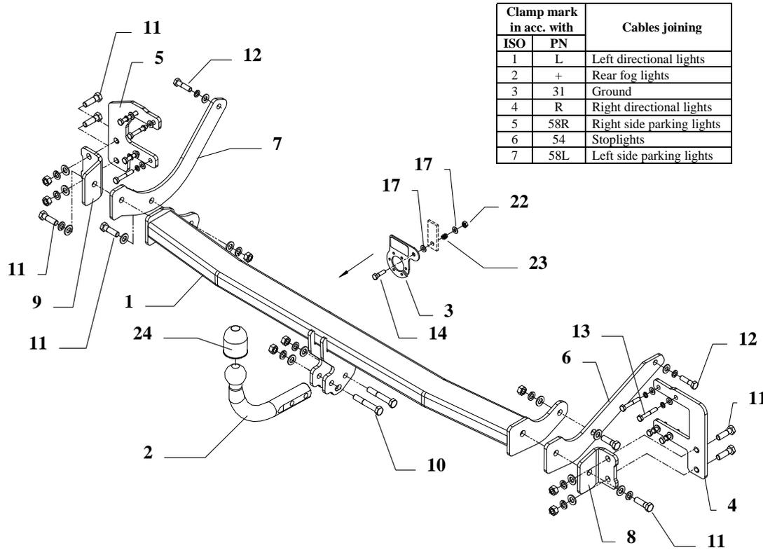
This towbar is designed to assembly in following car: **PEUGEOT 407 4 door**, produced since 2004 till 08.2008 (**Attention! Not suitable for car with 3.0 HDi V6 engine!**), catalogue number **F29** and is prepared to tow trailers max total weight **1900 kg** and max vertical load **65 kg**.
