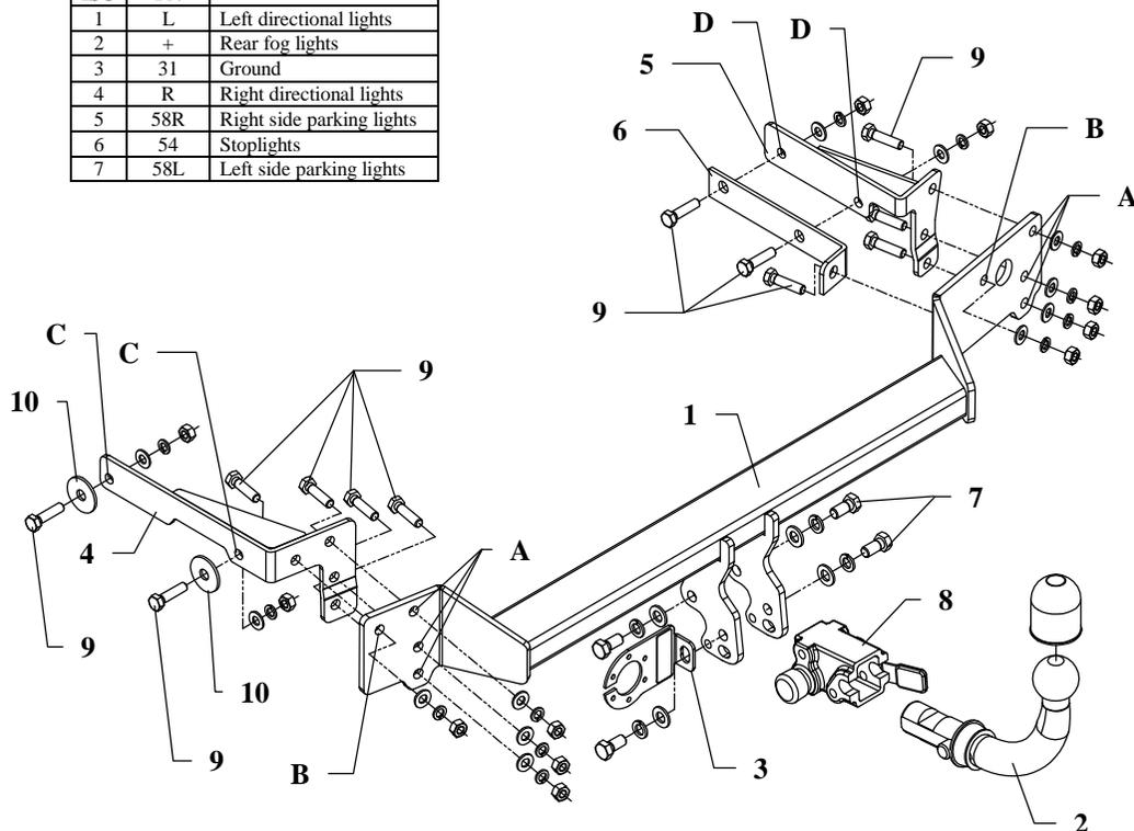
This towbar is designed to assembly in following car: **RENAULT CLIO B and C, 3/5 doors**, produced since 03.1998 till 09.2005 and **CLIO CAMPUS 3/5 doors**, produced since 2005 till 2010, catalogue no. **G29A** and is prepared to tow trailers max total weight **1200 kg** and max vertical mass **75 kg**.
