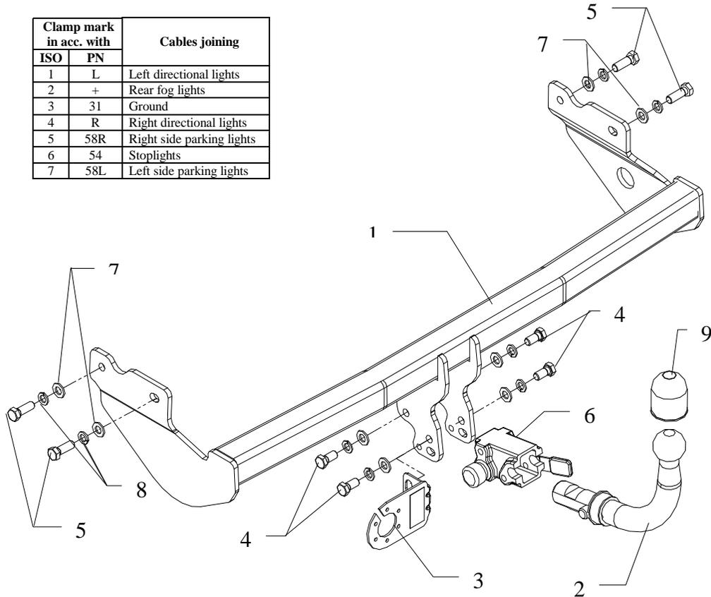
This towing hitch is designed to assembly in following car: **HYUNDAI GETZ**, produced since 2003 till 12.2004, catalogue number **J46A** and is prepared to tow trailers max total weight **1100 kg** and max vertical load **50 kg**.
