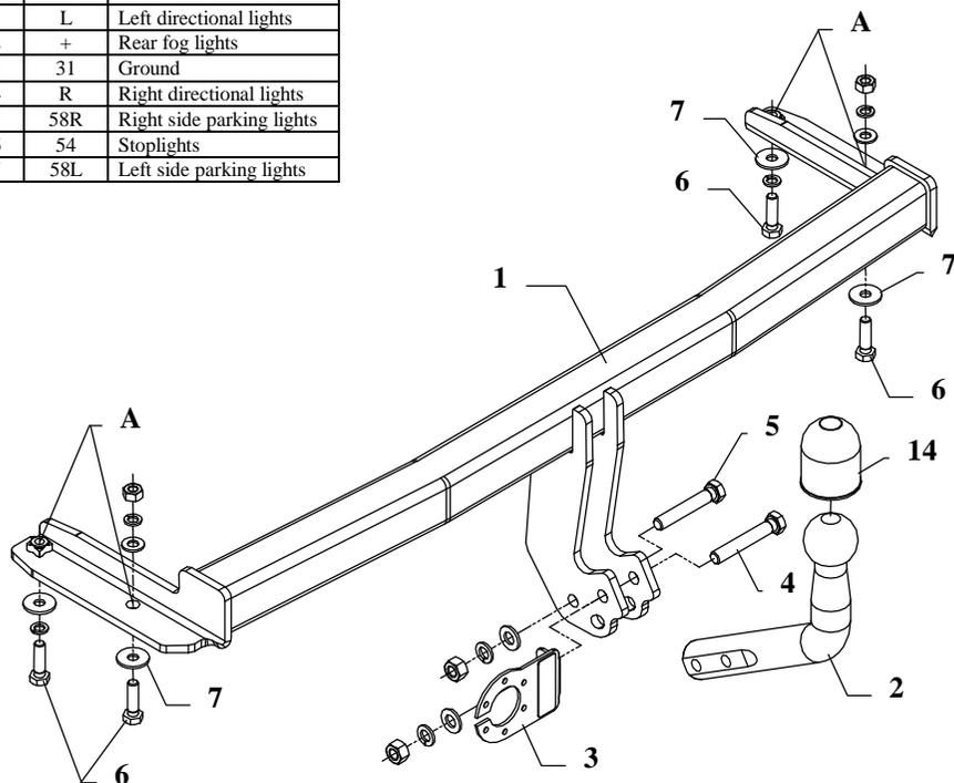
This towing hitch is designed to assembly in following cars: **SEAT IBIZA, 3/5 doors**, produced since 09.1999 till 04.2002, catalogue no. **SC03** and is prepared to tow trailers max total weight **1200 kg** and max vertical load **50 kg**.
