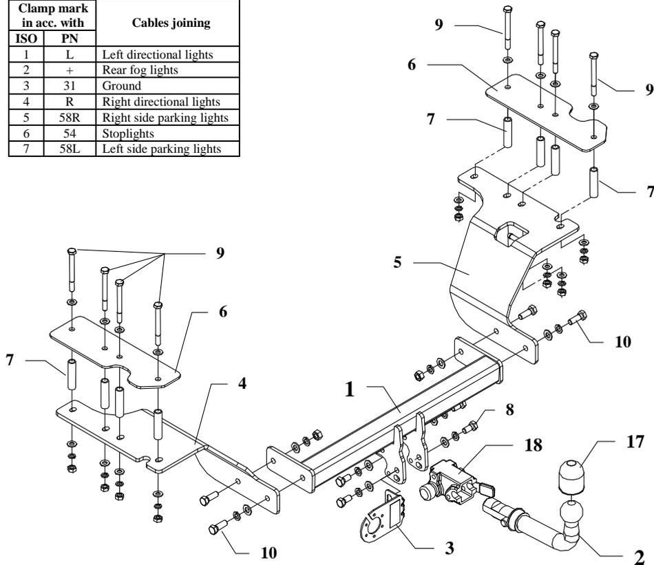
This towbar is designed to assembly in following cars: **HONDA CR-V** produced since 02.2002 till 02.2007, catalogue number **Y24A** and is prepared to tow trailers max total weight **1690 kg** and max vertical mass **100 kg**.
