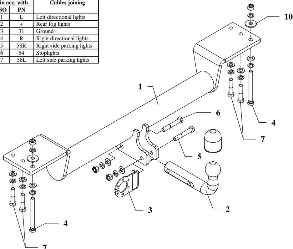
This towing hitch is designed to assembly in following cars: **MITSUBISHI PAJERO, V20, (V2/V4), 3/5 doors**, produced since 1991 till 2000, catalogue no. **Z02** and is prepared to tow trailers max total weight **3300 kg** and max vertical mass **135 kg**.
